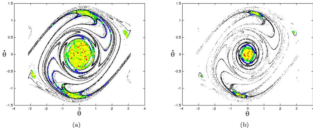
Figure 2: Contracted phase space for (2.2), with  $\alpha = 0.5$ ,  $\beta = 0.1$  and  $\gamma(t)$  decreasing linearly from  $\gamma_i = 0.05$  to  $\gamma_f = 0.02$  over a time (a)  $T_0 = 32\pi$  and (b)  $T_0 = 48\pi$ . The densities are coded with red being the most dense, then yellow, green, blue and black.
